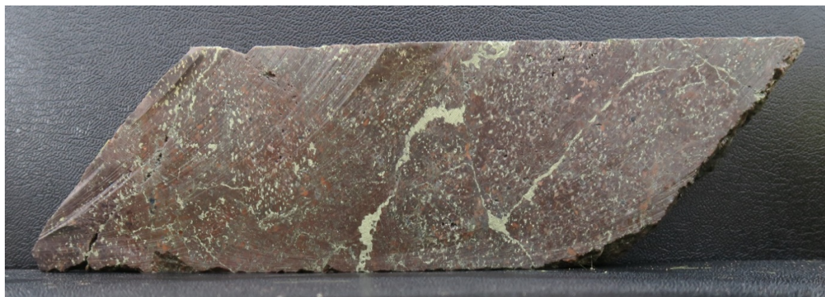
Figure 7.6 DCH-001, 346 m: Sulphide Zone: Abundant Disseminated and Veinlet Chalcopyrite and Bornite
