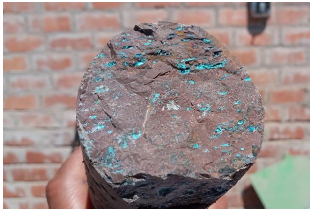
Photo 1. HQ core from DCH-074 with disseminated copper oxides in vesicles grading 1.4% Cu at 65 m depth
