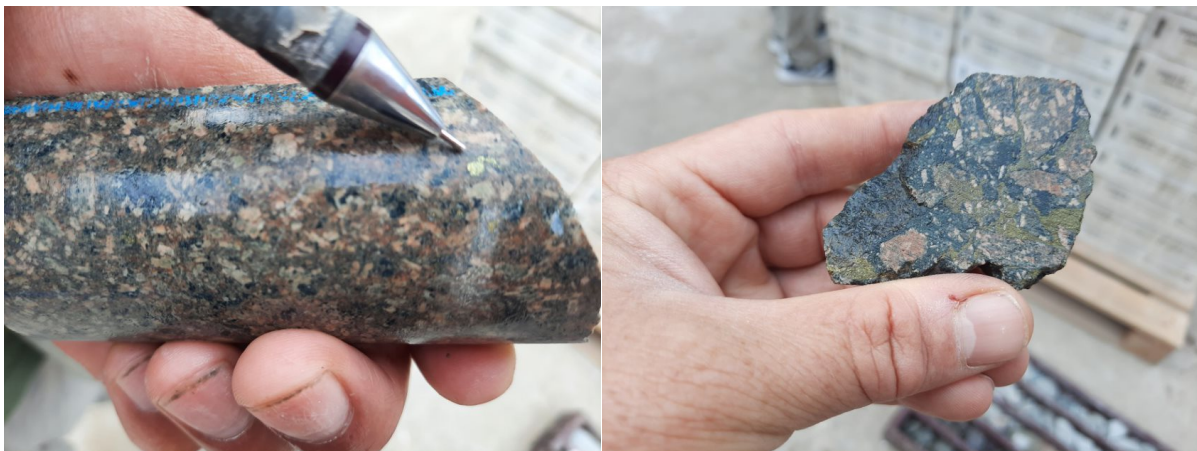
Figure 4. 2020 drill campaign. Chalcopyrite in hole DCH-072, interval 481.7-483.8m copper value up to 2.04% Cu
