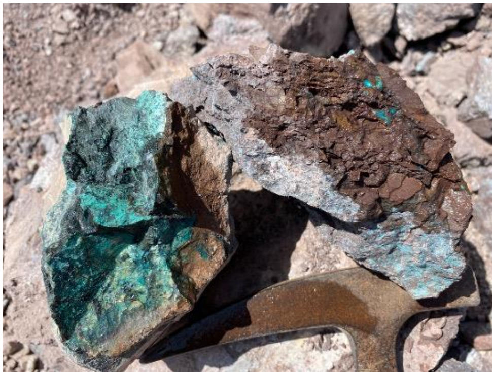
Picture 1. Rock containing oxidized copper uncovered during road construction at Lourdes Zone
