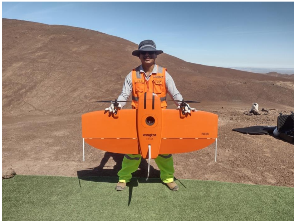
Picture 1. Topographic survey with WINGTRA Drone with high resolution image capture.
