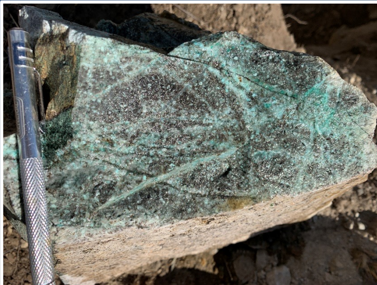
Andesitic porphyry with potassic alteration (biotite); quartz, A veinlets with albite cutting EDM veinlets; CuOx in fractures veinlets and disseminated
