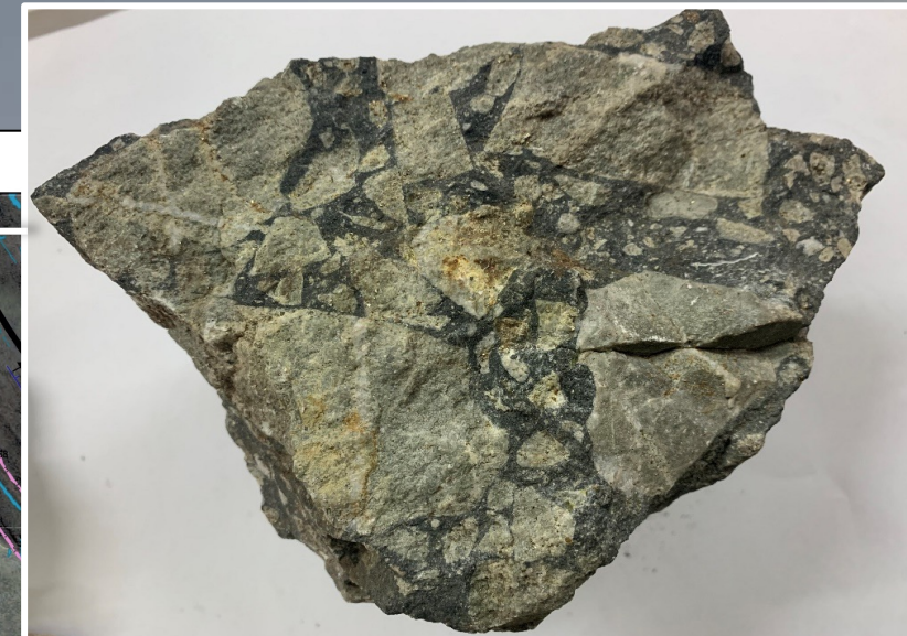
Tourmaline breccia, polimictic, clasts of sandstone and granodiorite porphyry with veinlets, quartz – sericite alteration, pyrite diss and molybdenum (weak)
