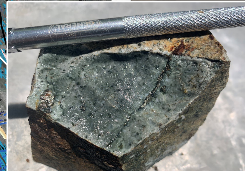
Andesite porphyry with actinolite-pyrite veinlet, also qtz milimetric veinlet, Feox in fractures; Calcopyrite in traces; 0.8 m wide, Quartz sericite alteration.
