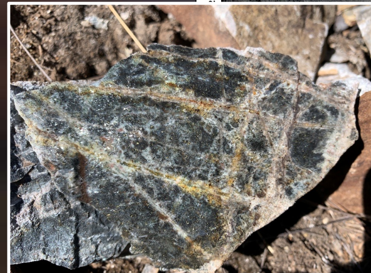
Dark rock, fine grain with stocwork , A, B, D type, biotite (weak), calcopyrite diss in parts.
