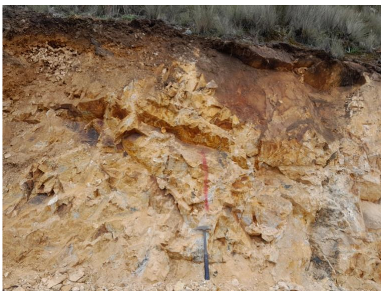
Figure 3. Yellowish-gray porphyry with moderate argillization, fine and thick quartz veinlets forming stockwork. The mineralization is represented by moderate black copper oxides in the fractures and in the vein walls.
