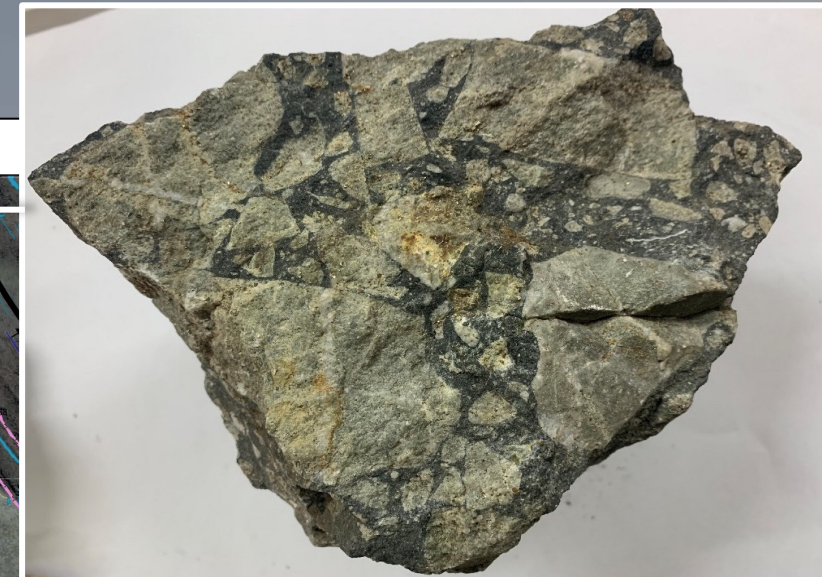
Tourmaline breccia, polymictic, clasts of sandstone and granodiorite porphyry with veinlets, quartz – sericite alteration, pyrite diss and molybdenum (weak)
