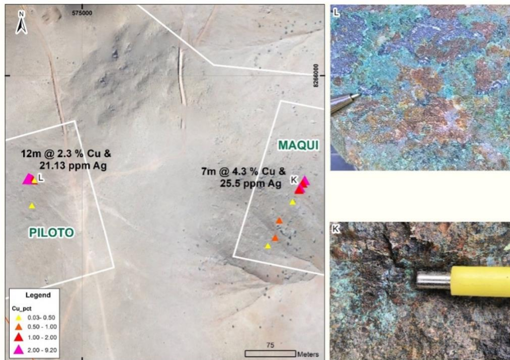
Figure 2. Highlights of copper channel results at L, K. The photographs show high-grade 2% to 4% copper oxides and sulfides such as bornite.
