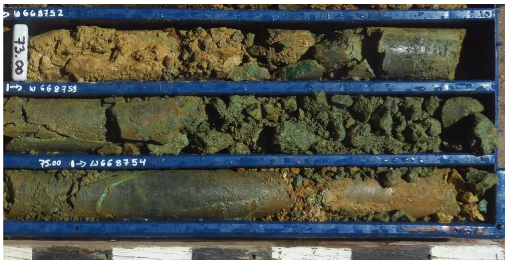
Picture 1. Example of high-grade copper mineralization in drillhole DCH-129. The 73 to 76-metre interval has an average grade of 2.13% copper.
